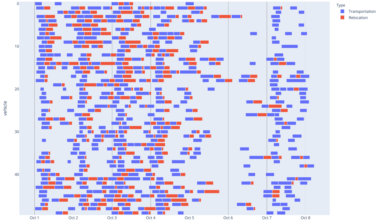
Figure 16: Autonomous Truck Schedule for the Large Network.
